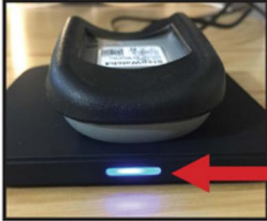
To charge StepWatch, place it face-down on the center of the charger.
