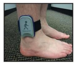
The StepWatch should rest just above the anklebone, on the outside of the leg.
