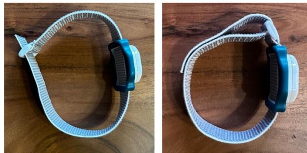
For StepWatch 5 without a buckle, fasten the Velcro side directly to the smooth side.
