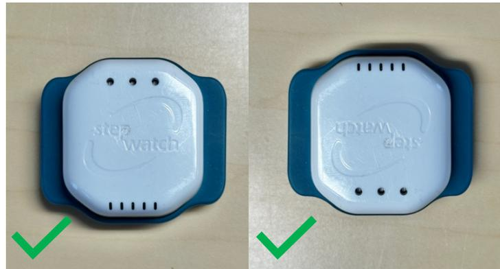
StepWatch 4 cannot be worn upside down. This will result in incorrect or missing data.
