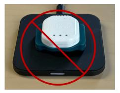
The StepWatch battery should last more than two weeks when fully charged. A flashing light on the charger inidcates charging error. If you see this, remove StepWatch, check connections, and place StepWatch back on charger. Light turns off when fully charged.
