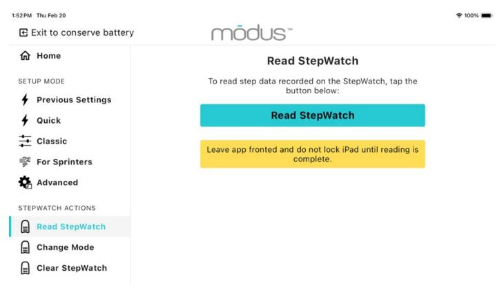
Tap "Read StepWatch" to begin the process. A progress bar will appear to indicate that data is being transferred. Be sure to keep StepWatch within Bluetooth range during the reading process.
