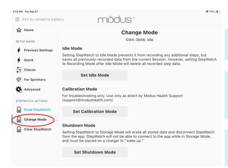
**Idle Mode** stops the recording of steps while saving all previously recorded data.
