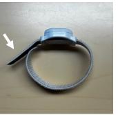
For StepWatch 5, fasten the Velcro side directly to the smooth side.
