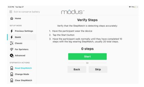
Quick Setup allows for only one verification. If StepWatch over- or under- counts by more than 10% (1 step), the algorithm is auto adjusted and setup progresses. If you want more tries to verify the settings, try using the Classic Setup option instead.
