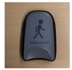
The StepWatch can be worn over a sock and can be worn on either leg, but it needs to be worn on the outside of the leg and facing upright. See "Managing a StepWatch" for additional notes on wearing and maintaining the StepWatch and associated parts
