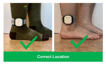
StepWatch 4 <u>cannot be worn upside</u> <u>down</u>, or on the inside of the ankle. This will result in incorrect or missing data. StepWatch 5 can be worn upside down, but must be worn on the outside of the ankle.
