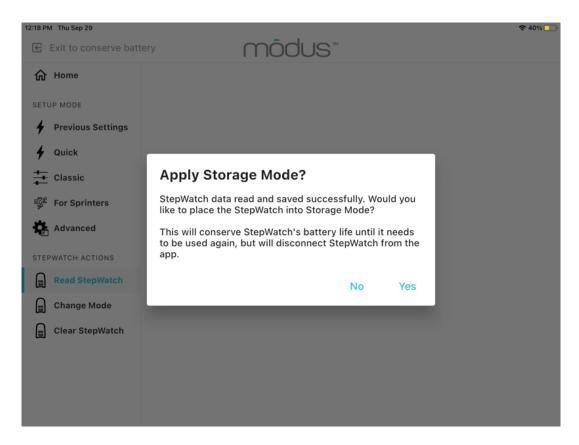
Selecting "Yes" turns off the Bluetooth radio. Select "Yes" if you will not be using this StepWatch again immediately and wish to conserve its battery. You will have to wakeup the radio when you want to use this StepWatch again by charging it for at least 10 seconds before connecting to it.
