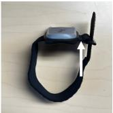
For StepWatch 4, pull the strap through the plastic ring and secure using the Velcro tip.
